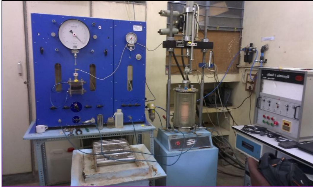
cyclic triaxial setup
